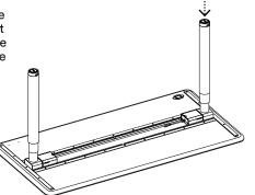
3. Insert the knob on the control box through the notch in the chassis and slide to the right.
