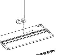
2. Align the knobs inside the foot with the notches on the leg cap. Rotate the foot 90° until you hear the click of the release button. (To remove the foot, press the release button.)
