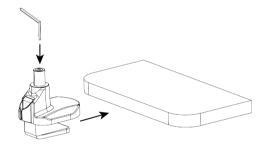
2. Slot the monitor arm onto the base and use the allen wrench provided to tightly pin the arm to the base.
