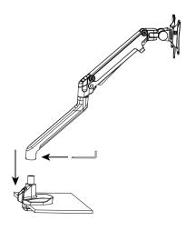
3. Install two monitor mounting screws into your monitor using the allen wrench. Carefully hang the monitor on the monitor mounting plate, engaging the two holes that best align to the monitor screws. Install the remaining monitor mounting screws in the lower half of the mounting plate using the allen wrench.
