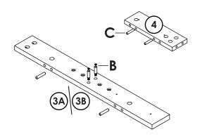
Install cam lock pins into framework
